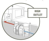
Our high-level discharge is equipped with a reliable, high quality, pump kit. This kit is delivered pre-assembled for ease and speed of installation. Intermittent operation by float switch.
